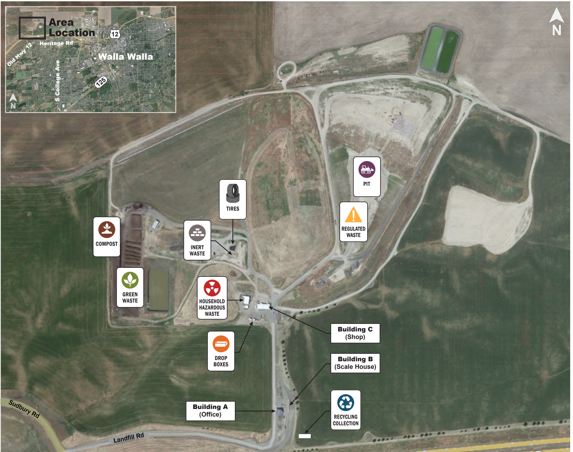
Figure 5-1. Sudbury Road Landfill: Existing Site Layout
